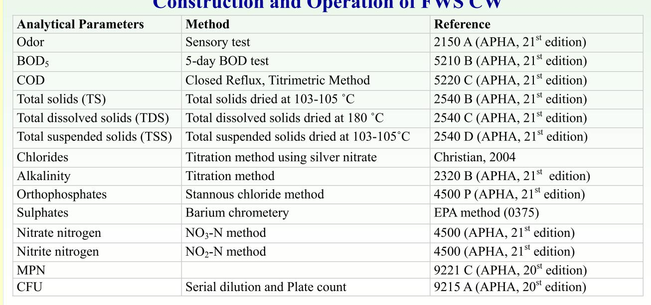
**Physico-chemical and Microbiological characterization of waste** water after 2.5 hr HRT (continuous mode) through FWS CW
