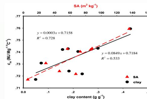
Fig. 1 Specific heat of soil minerals ( $c_m$ ) as related to specific surface area (SA) and clay content of the samples.
