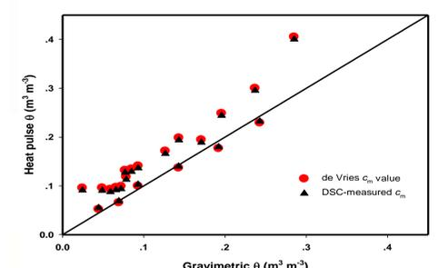
Fig. 3 Comparison of the heat-pulse  $\theta$  (with  $c_m$  of 0.725 MJ Mg<sup>-1</sup> °C<sup>-1</sup> and  $c_m$  from DSC) versus gravimetric  $\theta$ .
