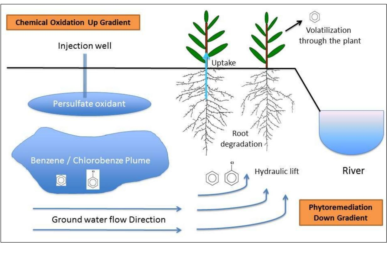
Fig. 1. The remediation plan to use Persulfate Oxidation and Phytoremediation to clean up benzene compounds in a former pesticide plant in Southern Brazil.
