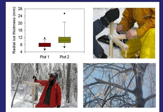
**Ice Accumulation:** Average radial ice thickness was 7.8 mm (±0.4 SE, n=19) in Plot 1 and 11.6 mm (±1.3 SE, n=14) in Plot 2. This compares to 5.9 to 14.4 mm during the 1998 ice storm event at the site.
