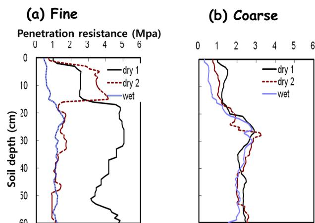
Fig. 1. Penetration resistance according to the soil moisture condition and soil texture
