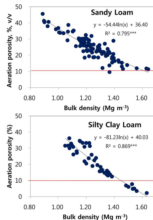
Fig. 3. Relationship of bulk density and aeration porosity for silty clay loam and sandy loam (p<0.01).
