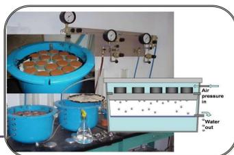
◆ Experiment 1. Assess of soil compaction effect on pressure by using apparatus designed for compaction; disturbed
