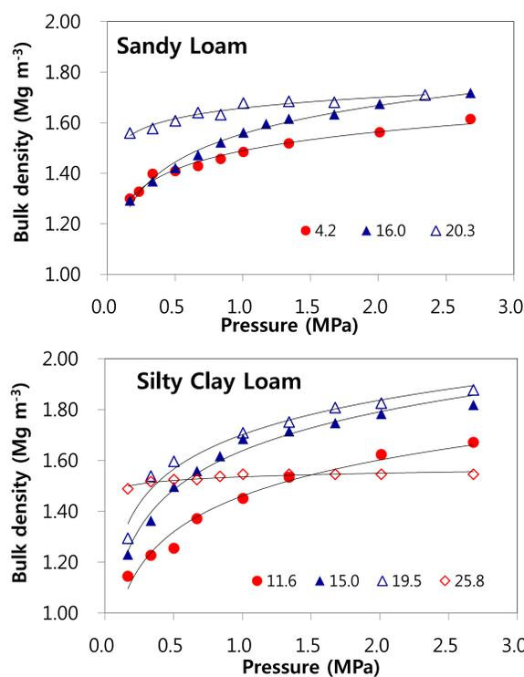
Fig. 2. Relationship of pressure and bulk density for silty clay loam and sandy loam according to soil water contents (p<0.01).
