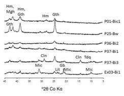
Figure 1. XRD patterns - oriented clay of soils from ferruginous dolomite of the Gandarela formation (Hm: hematite, Mgh: maghemite, Gth: goethite, Cln: kaolinite, Tdq: todorokite, Mic: mica, Lit: lithioforite, Gb: gibbsite)
