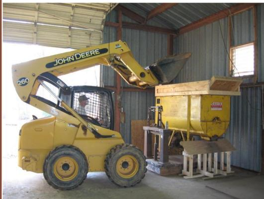
Broiler litter with or without alum (20% by litter weight) was mixed in a feed mixer and stacked in individual wooden bins (1.2 x 1.2 x 1.2 m)..
