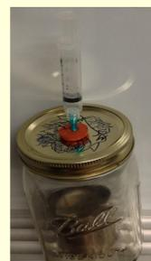
Fig 4. Soil incubation vessel. Air samples were taken with a syringe, stored in glass vials and analyzed for CH<sub>4</sub> using gas chromatography (FID – flame ionization detector)
