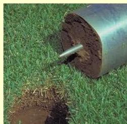
Fig 2. Intact soil core for determination of diffusion coefficients
