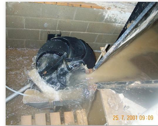
H-Flume and Coshocton Wheel Sampler
