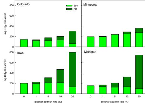
Figure 2: Cumulative SOC-derived and biochar-derived respiration over the 2 years of laboratory incubation for the 4 soils and the 5 biochar addition rates.
