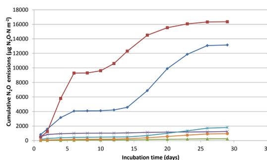
Figure 1 The  $N_2O$  flux and cumulative  $N_2O$  emissions under different soil moisture conditions. There is a shift from nitrification to denitrification around 70% WFPS.
