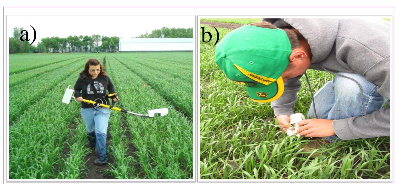
Figure 1: Diagnostic tools used for predicting protein content: a) Greenseeker Model 505; b) CCM-200 Chlorophyll meter. Measurements taken at the Zadoks GS 16.
