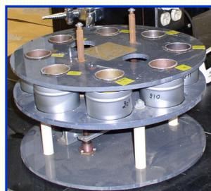
Fig.2 Standard Wet-sieving Machine
