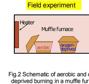
Fig.2 Schematic of aerobic and oxygen-deprived burning in a muffle furnace.
