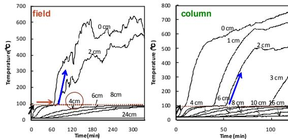
Fig.3 Soil temperature during surface burning
