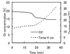
Fig.1 Temperature and oxygen concentration during surface burning.
