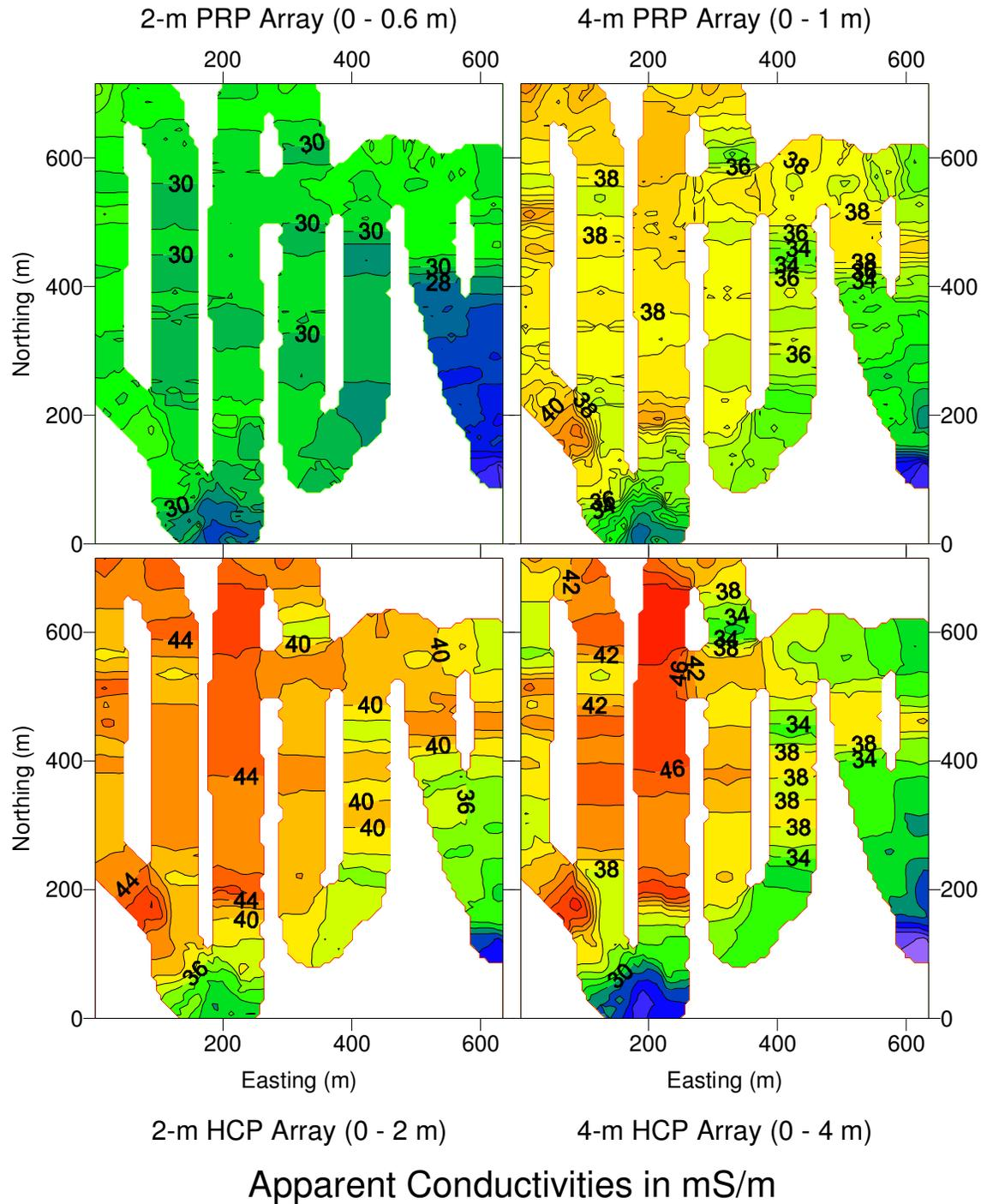
**Figure 5:** Apparent Conductivities on Freshwater Lagoon.
