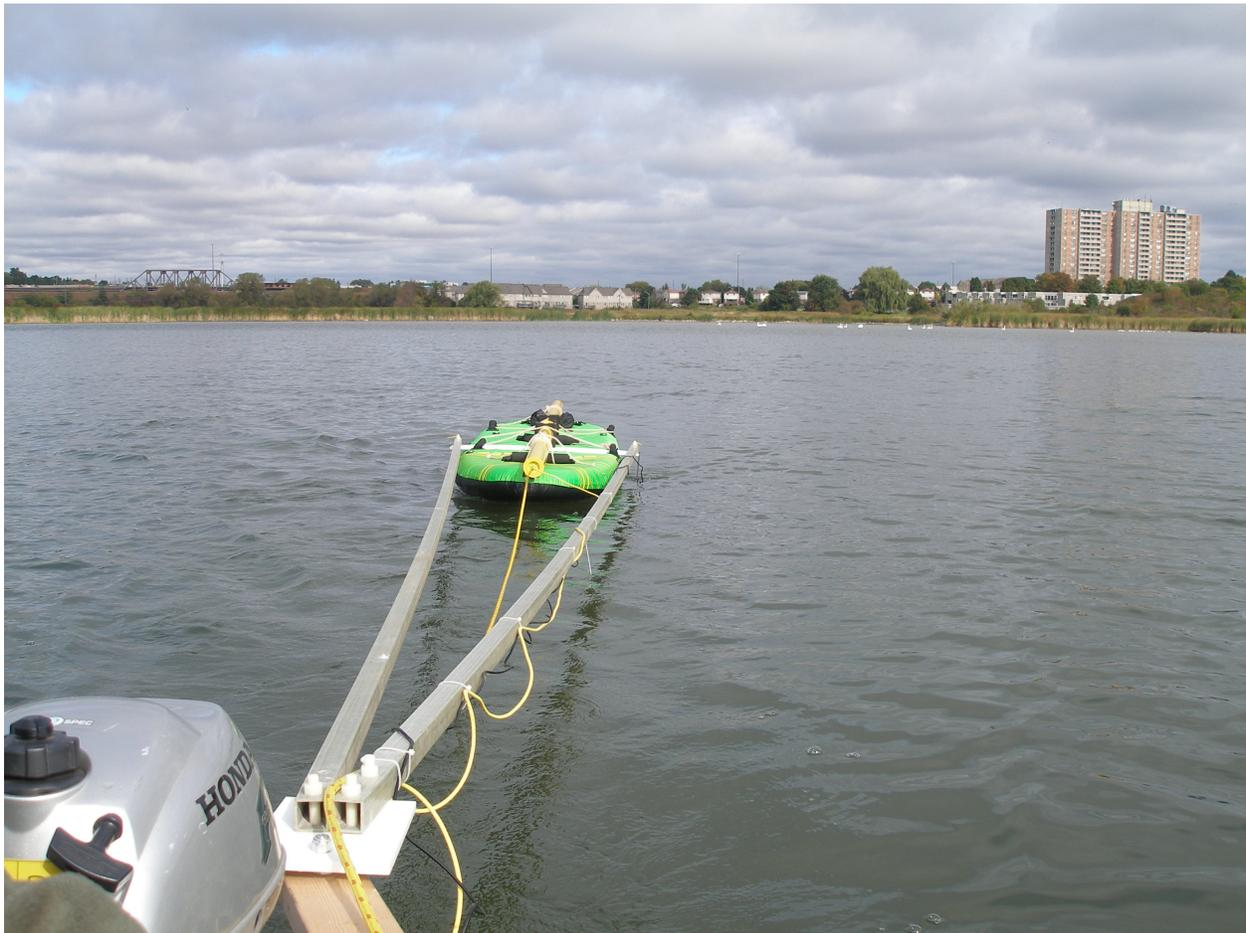
**Figure 2:** EM Instrument with 4-m and 2-m HCP- and PRP-Arrays. (Photo: D. Lalonde)
