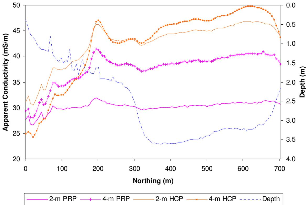
**Figure 6:** Apparent Conductivities and Water Depth along 200 E.
