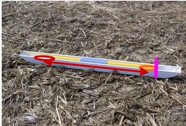
**Figure 1:** EM Instrument with 1-m HCP- and PRP-Arrays. (Photo: Dr. B. Allred)
