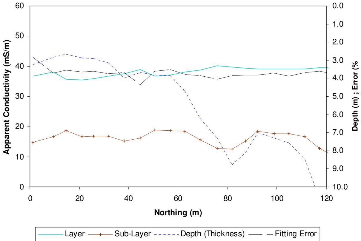
**Figure 8:** Estimated Conductivities and Depth, with Estimation Error for Portion of 200 E.
