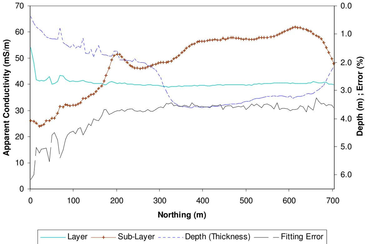
**Figure 7:** Estimated Conductivities, Water Depth and Estimation Error along 200 E.
