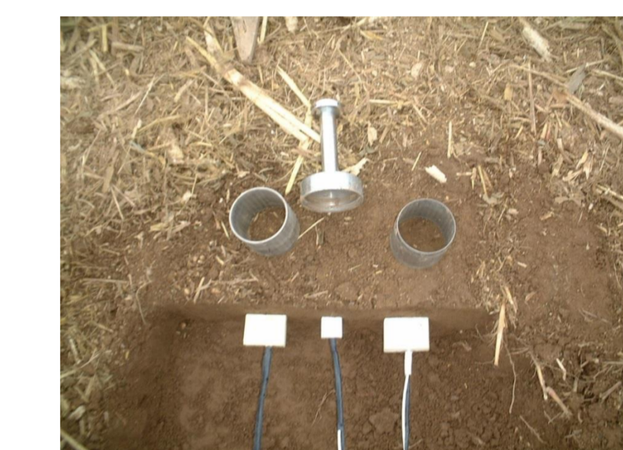
Fig 2. Field installation of standard and improved thermo-TDR probes in the NT treatment. Cylinders are for soil cores.
