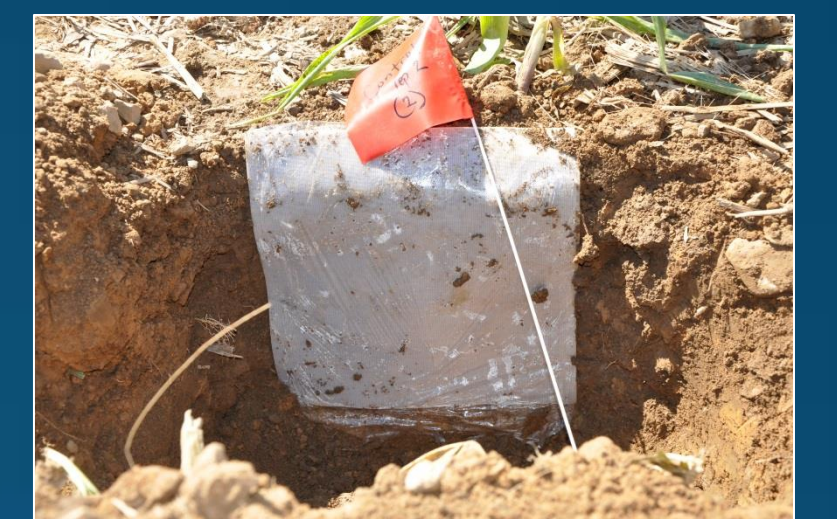
Resin sheet after soil excavated
