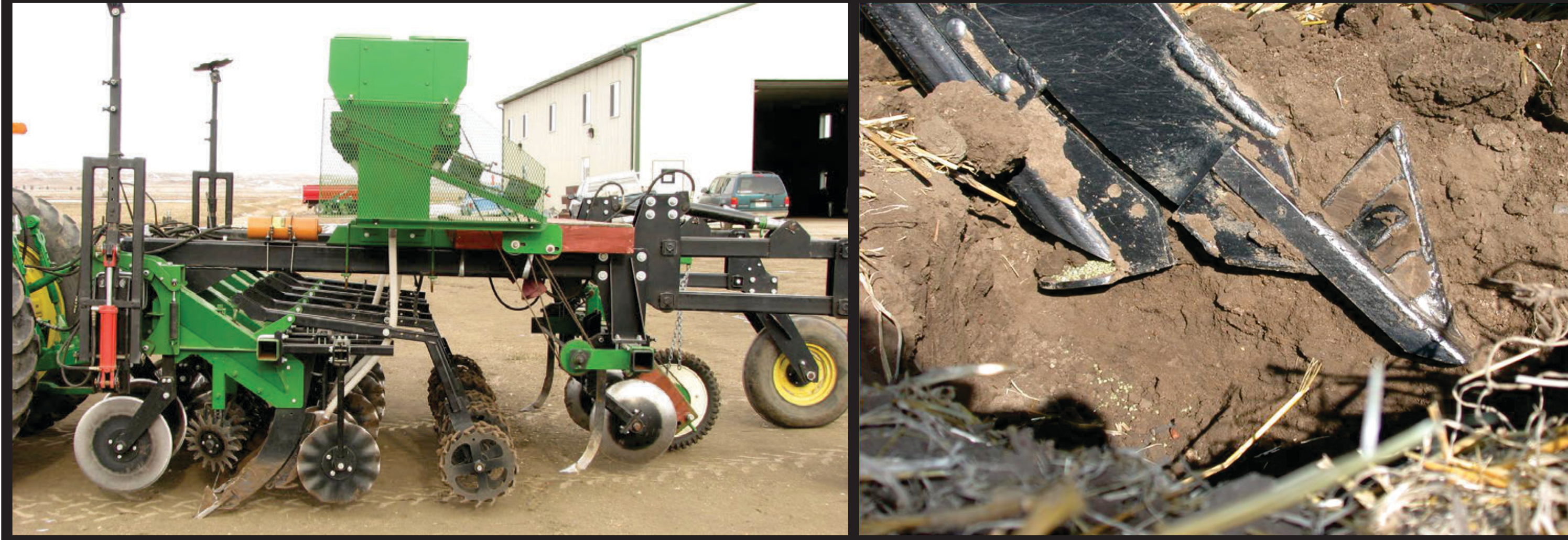
Figure 1. (Left) Modified six-row strip till implement used for evaluation of PCU in a study conducted near Williston ND from 2008 through 2011. Row spacing was 60 cm and tillage depth was approximately 25 cm. Figure 2. (Right) Tillage shank with fertilizer delivery tube attached to the back.
