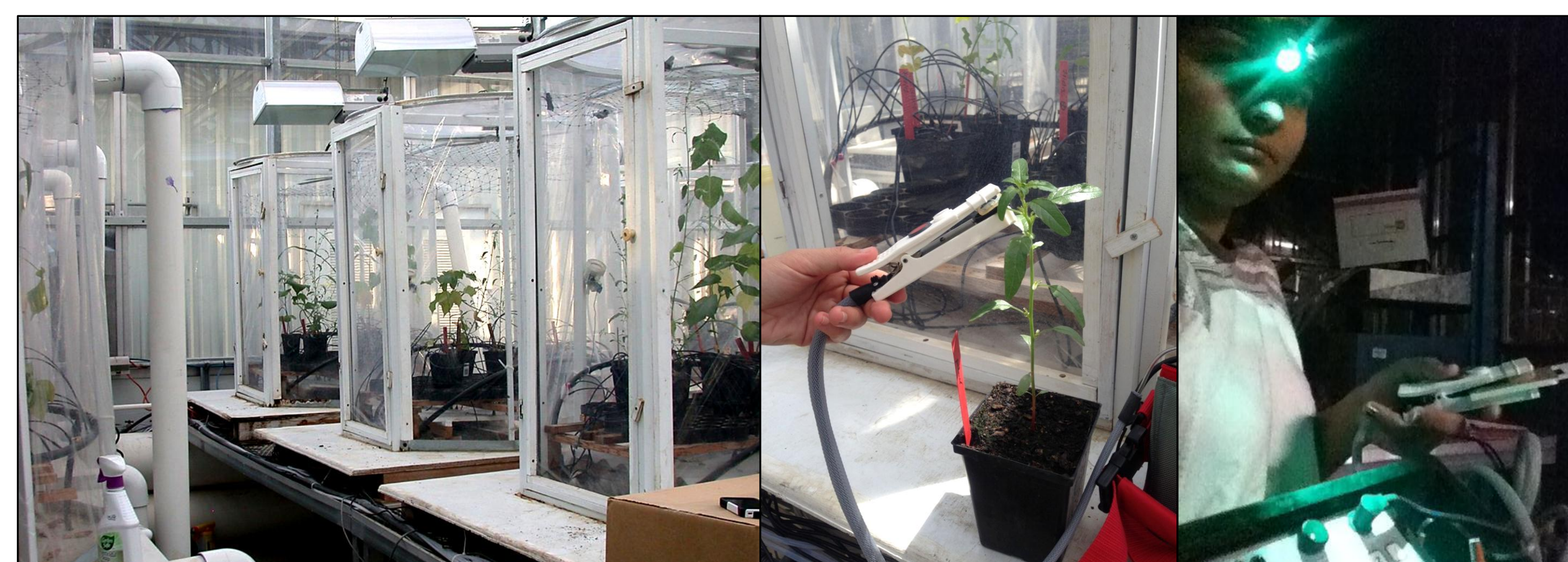
Fig. 1. Plants growing in the chambers (L), and day-time (C) and night-time (R) stomatal conductance measurements on the plants.
