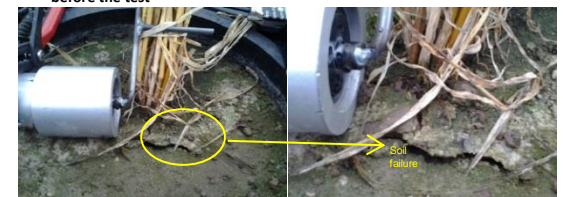
Fig. d (b, c) Plant pushed with the lodging arm to 45° from vertical axis and soil failure occurred
