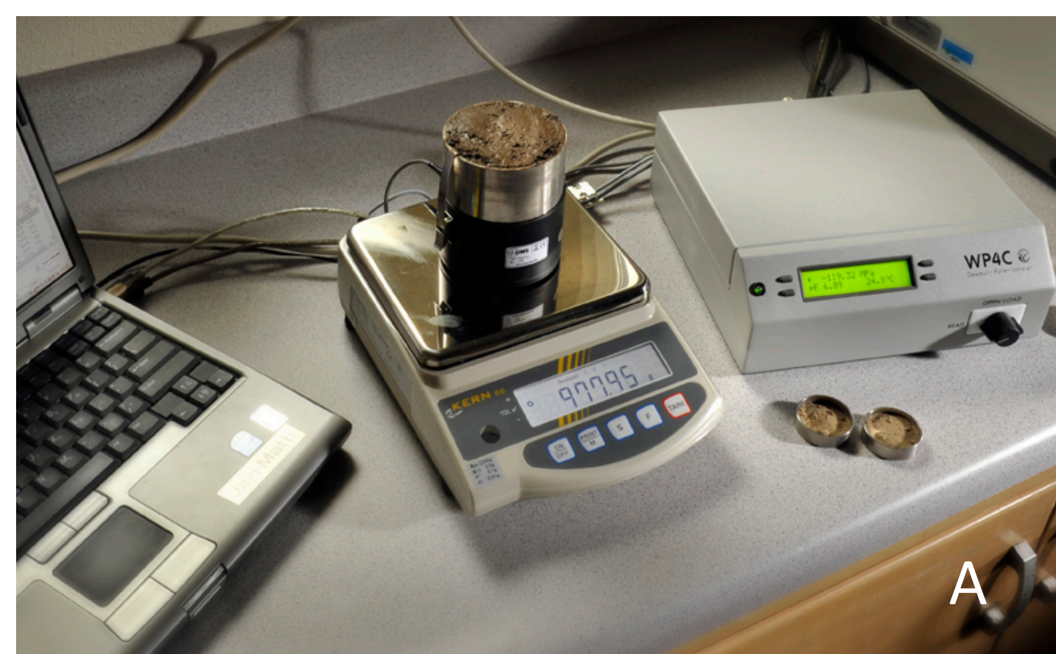
Figure 1. A.) Instrumentation used in this study. Hyprop automated SMCC generator from UMS (center) and WP4C dewpoint hygrometer from Decagon (right). B.) Cutout of the Hyprop showing placement of the two tensiometers in the soil.
