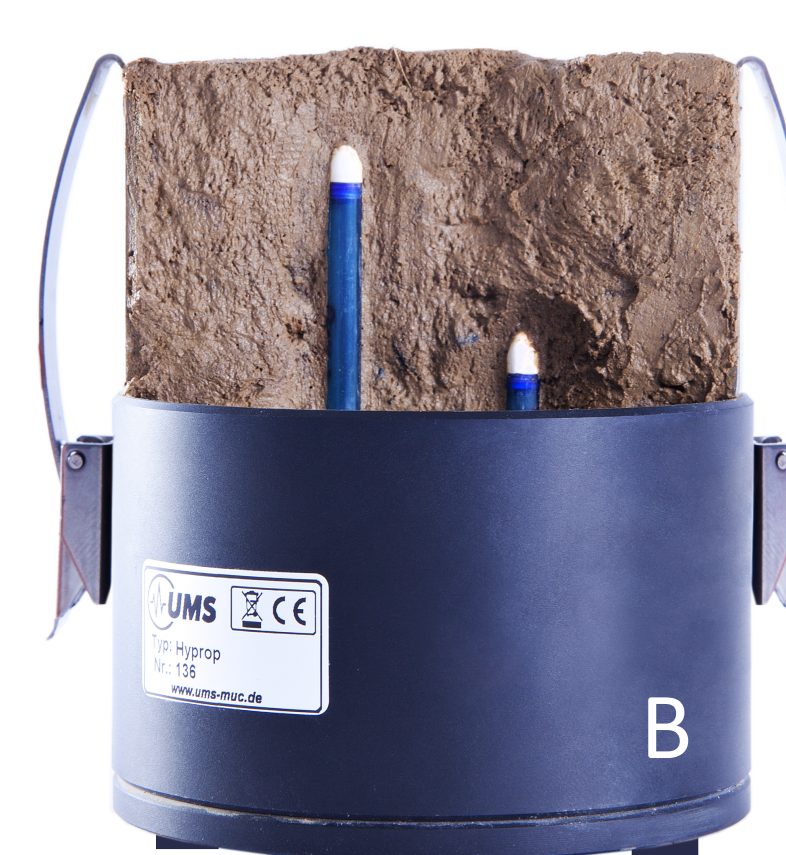
Figure 1. A.) Instrumentation used in this study. Hyprop automated SMCC generator from UMS (center) and WP4C dewpoint hygrometer from Decagon (right). B.) Cutout of the Hyprop showing placement of the two tensiometers in the soil.
