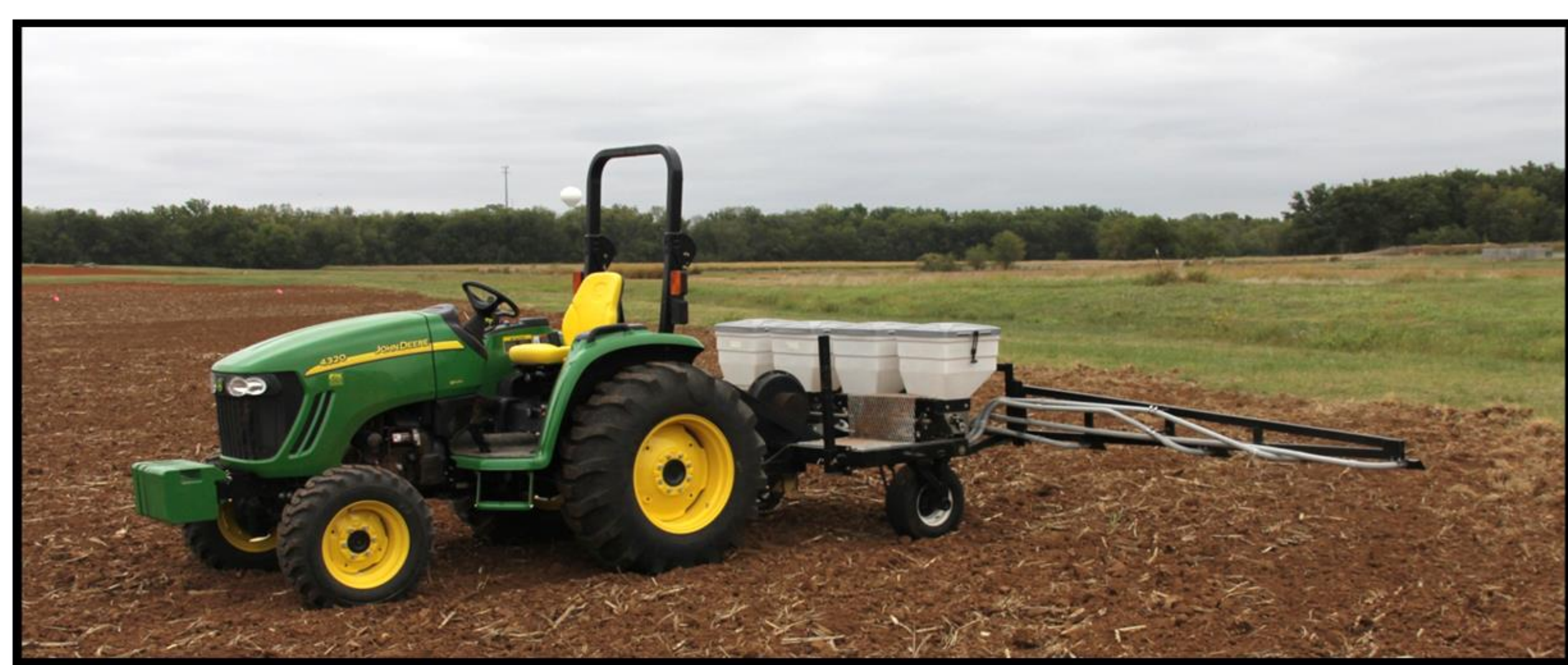
Figure 1. NPKS Applicator built by OSU Ag Engineering. Applicator used a PTO driven fan to blow fertilizer down boom and ground driven Gandy boxes to control fertilizer flow rate.
