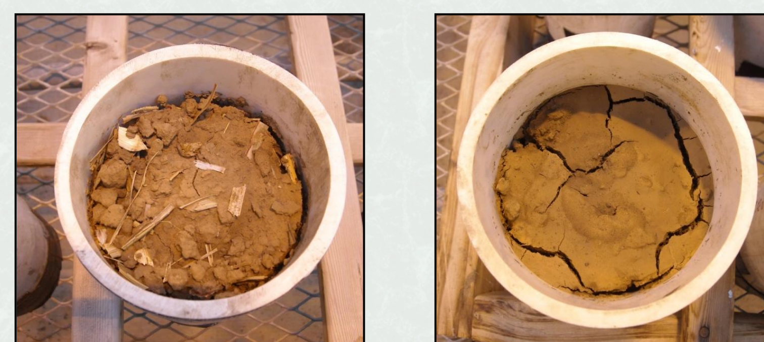
Above: (Left) PVC column with residue (+R), and (Right) PVC column without residue (-R).
