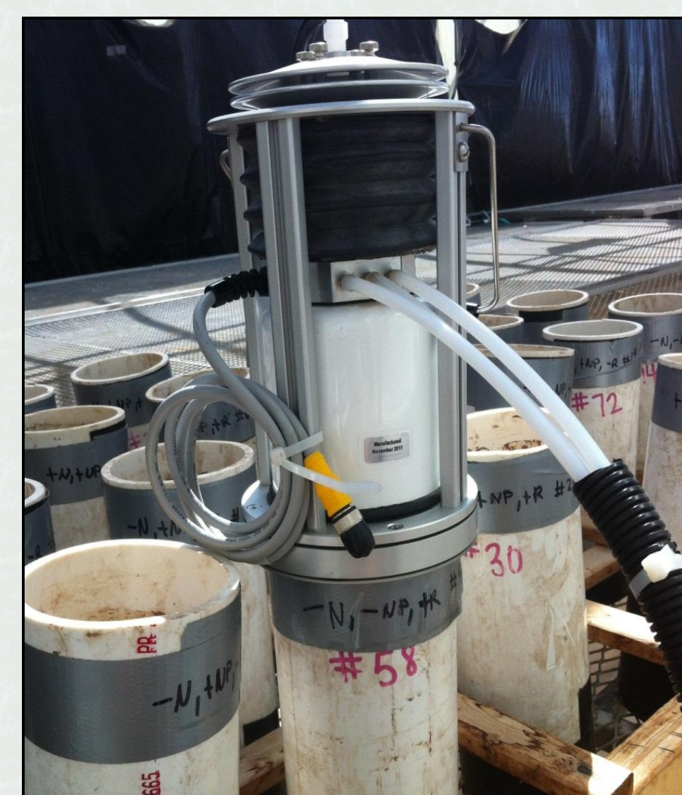
Above: Li-Cor chamber atop a PVC treatment column
