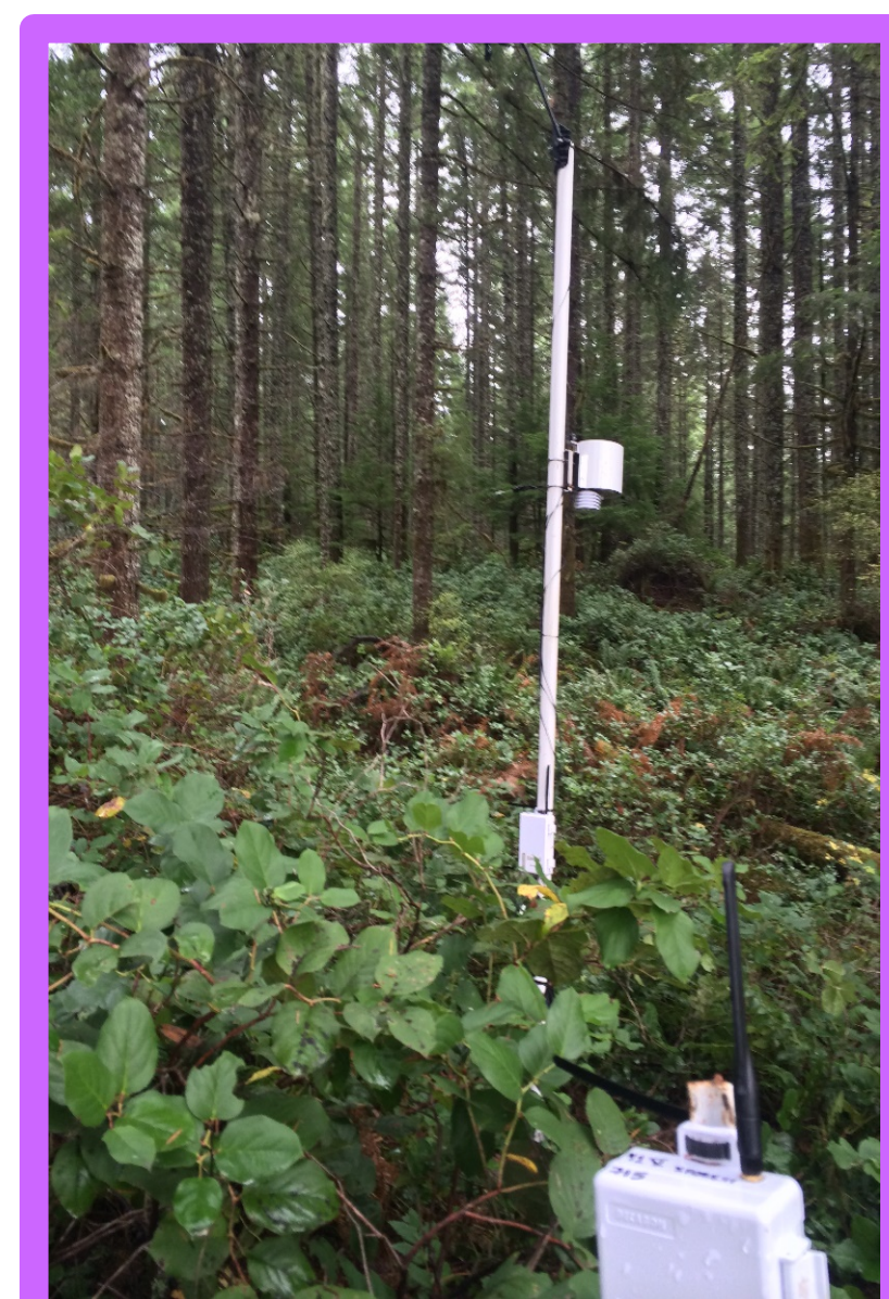
Decagon data logger in the foreground and Decagon weather station including an anemometer, solar radiation, leaf area wetness, relative humidity, air temperature, relative humidity sensors and a tipping bucket rain gauge. Data collected on the treated and reference stand every hour. Untreated forest stand.
