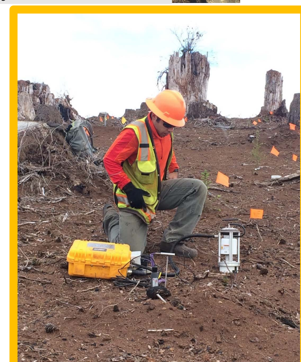
LiCOR (yellow) infrared-CO 2 device placed on a PVC collar (white). Soil moisture probe (grey) and soil temperature probe (purple) used for each observation. Data collected monthly, on nine known locations per plot. Efforts were also made during summer to identify a diurnal pattern in soil respiration. Treatment E.
