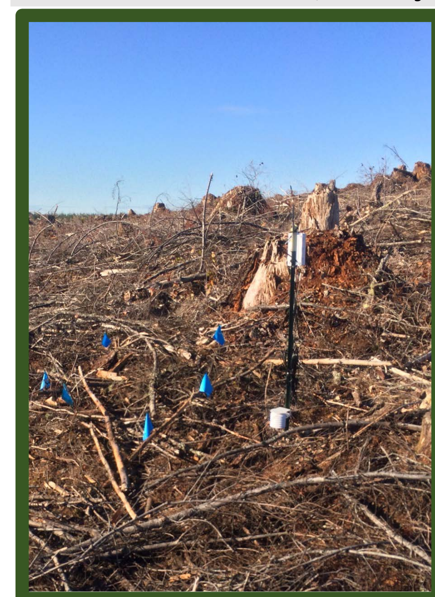
Decagon data logger connected to soil moisture/temperature probes at 10, 20, 30, & 100cm depth. Air temperature and relative humidity also at 15cm above mineral surface. Data collected hourly on all plots. Treatment A.
