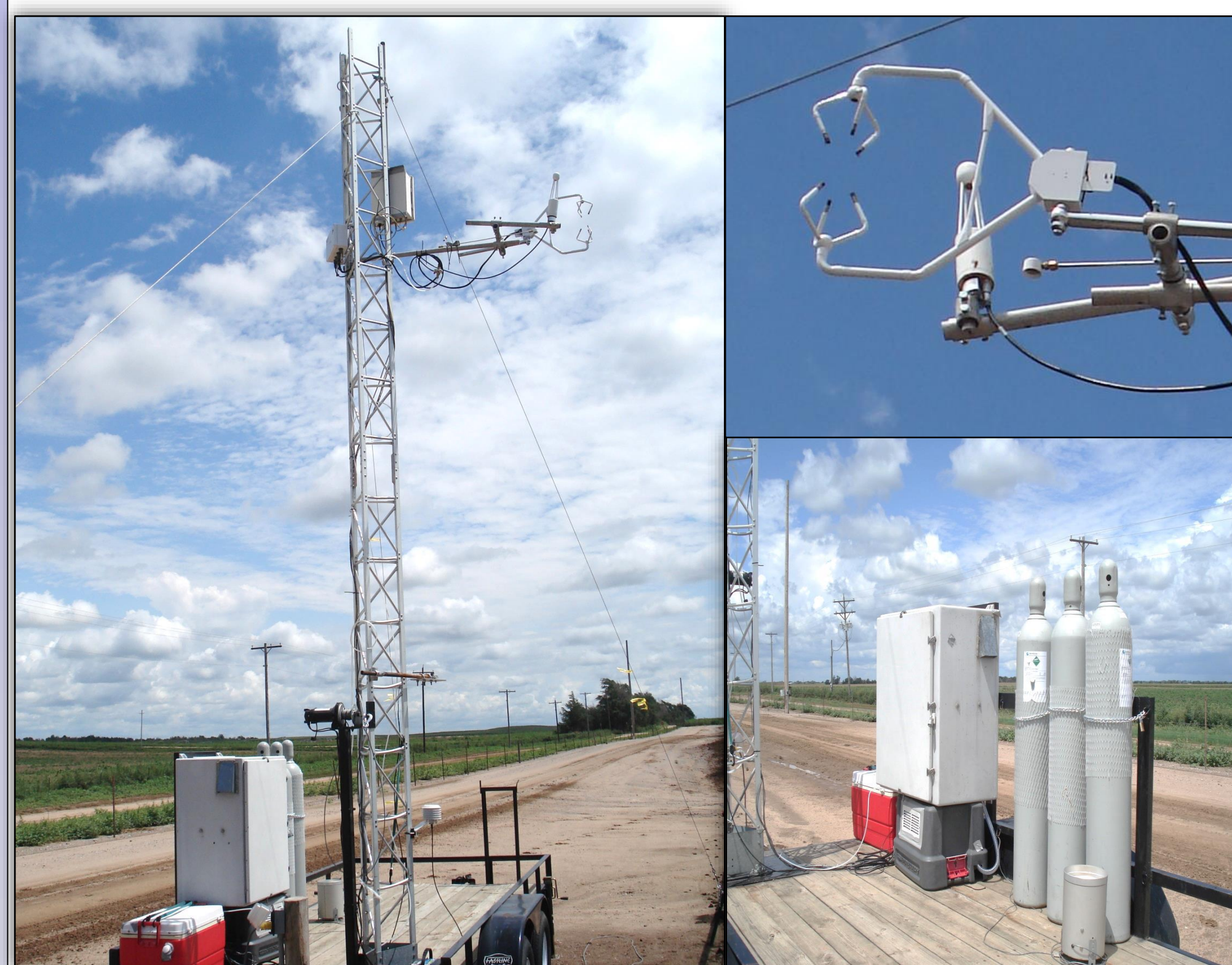
Instruments: Open-path, Closed-path, Data loggers, Sonic Anemometer (Campbell Scientific).
