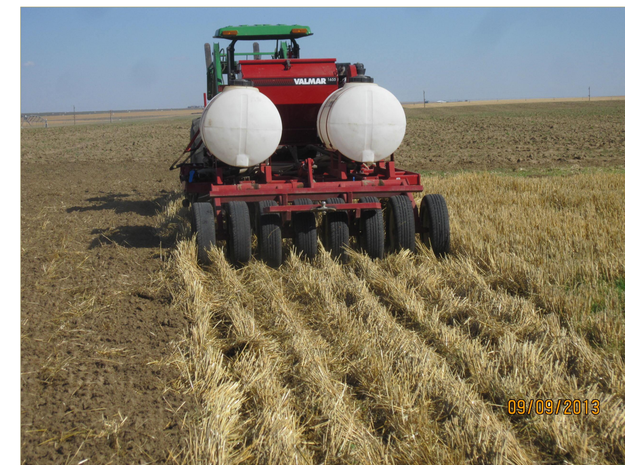
Fig. 2. Direct seeding winter canola into newly-harvested winter wheat stubble. The drill is equipped with hoe openers spaced 12-inches apart with openers staggered on three ranks to enhance residue clearance. This drill was used to plant all (except for the broadcast) treatments in the experiment.
