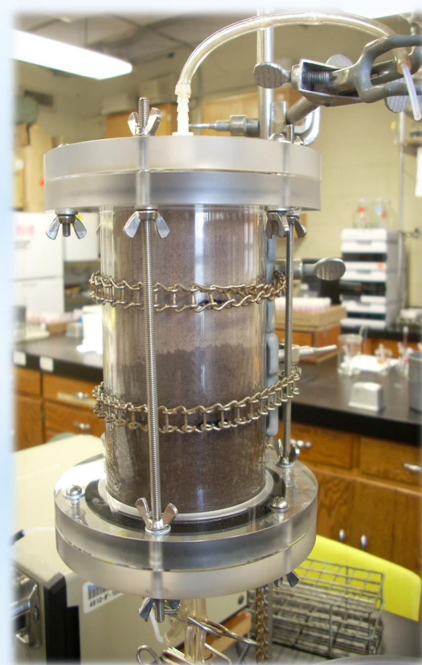
Fig.1. Soil Column Showing Wetting front During Bh Horizon Saturation. Photo: J. Leiva
