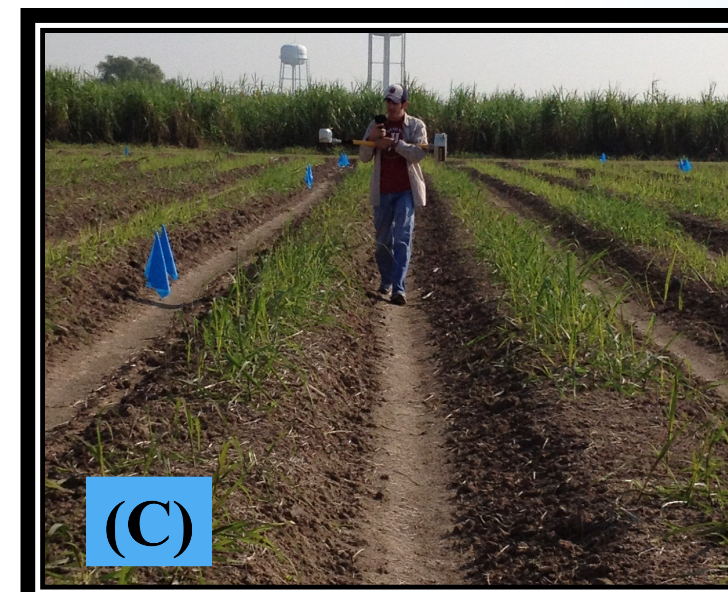
Pictures (A-D): (A) Mechanical planting of energy cane billets; (B) Knifing-in of liquid N fertilizer (as urea ammonium nitrate); (C) Collection of canopy reflectance reading using GreenSeeker® handheld sensor two months after emergence and (D) at maximum tillering stage
