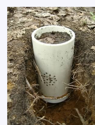
Zero-tension lysimeters installed underneath soil mesocosms to collect gravimetric soil water
