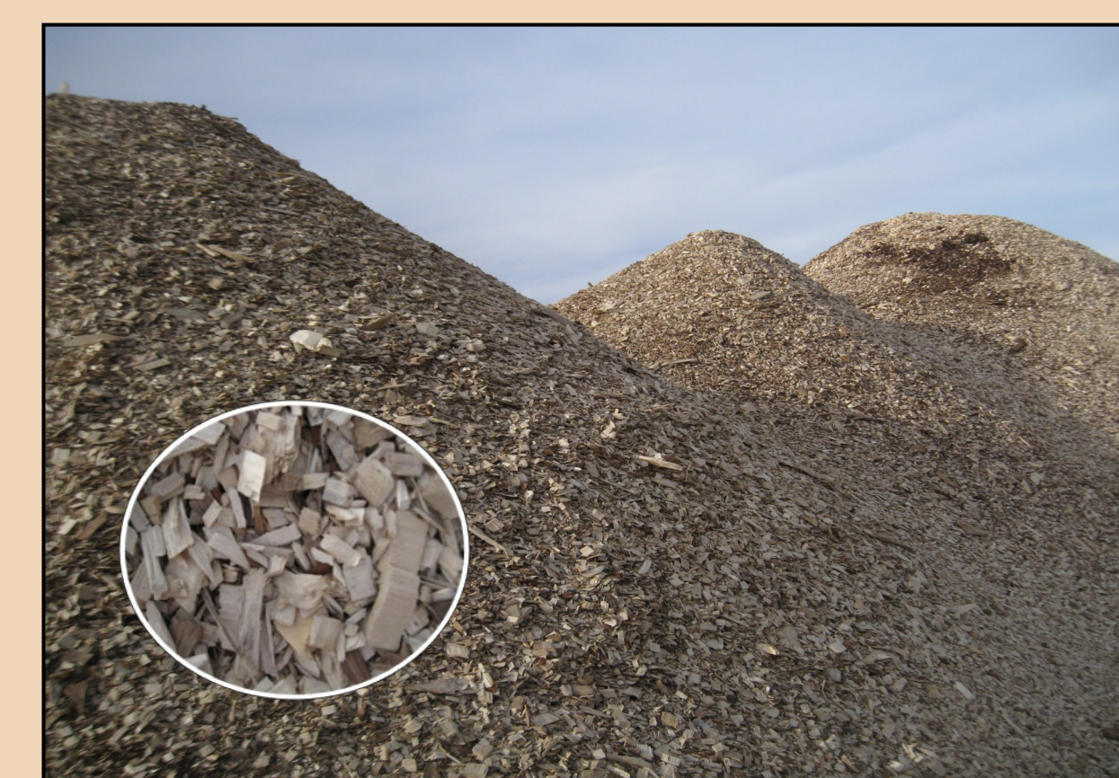
2. Woodchips used as a carbon source for denitrifying bacteria in the bioreactor.
