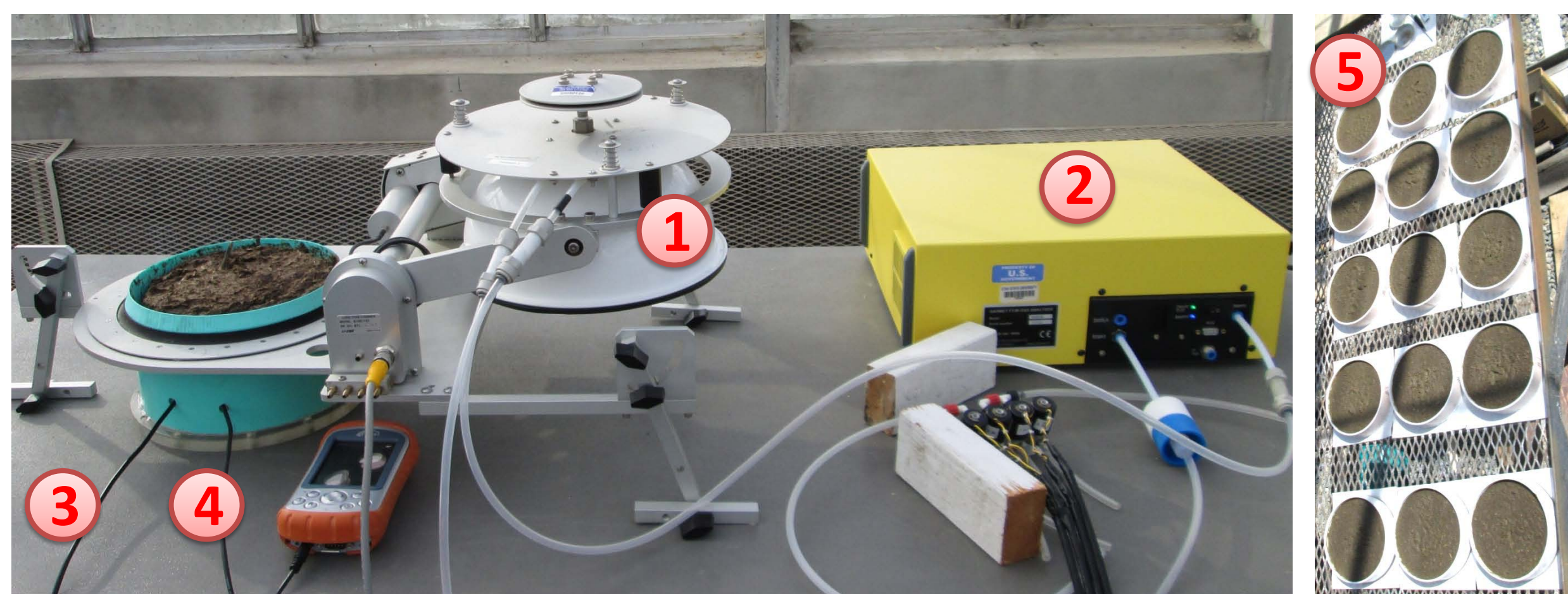
Fig. 1. Experimental Facility. 1 – Dynamic closed Chamber, 2 – FTIR, 3 – moisture sensor wire, 4 – thermistor wire and 5 – samples for chemical analysis.
