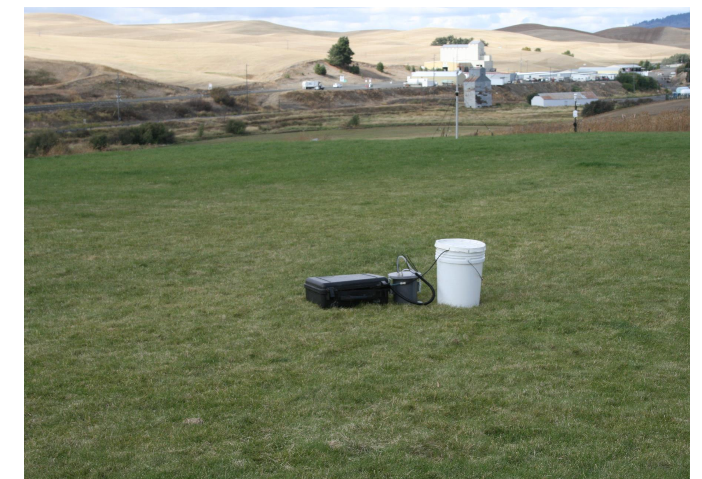
Figure 2. Testing infiltration on the soccer field.
