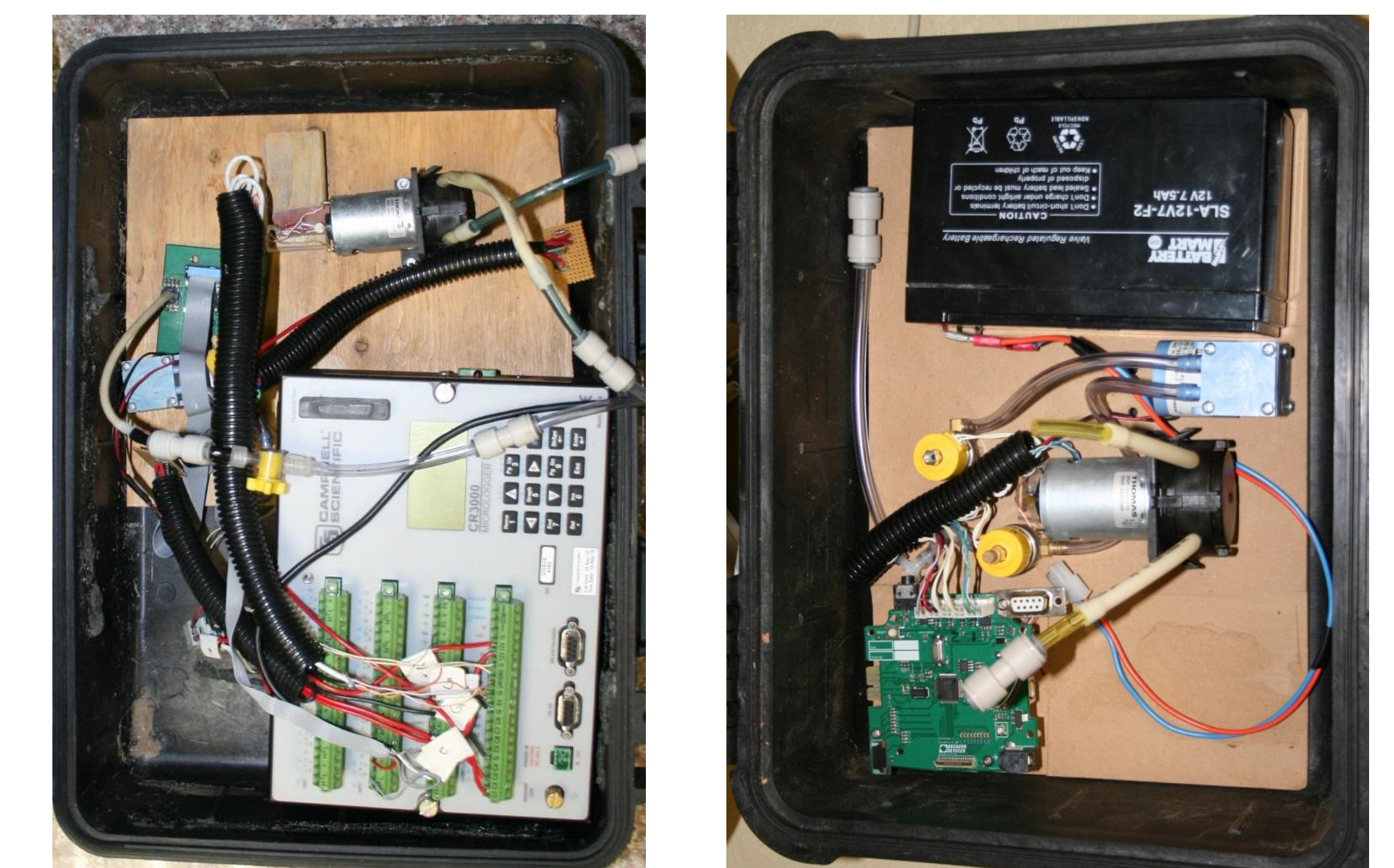
Figure 1. Internal layout of infiltrometer. On left is original prototype with data logger. On right is second edition with purpose built board.
