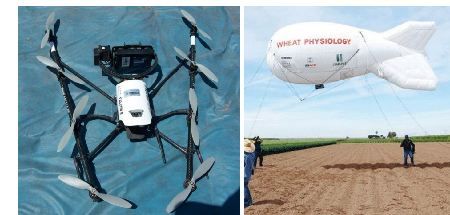
Left: The multi-spectral camera, measuring in the spectral range of 400 – 900nm, attached to a UAV. Right: The helium filled blimp taking measurements of a field trial in Obregon, Mexico. Image courtesy of http://blog.cimmyt.org/?p=7892 .
