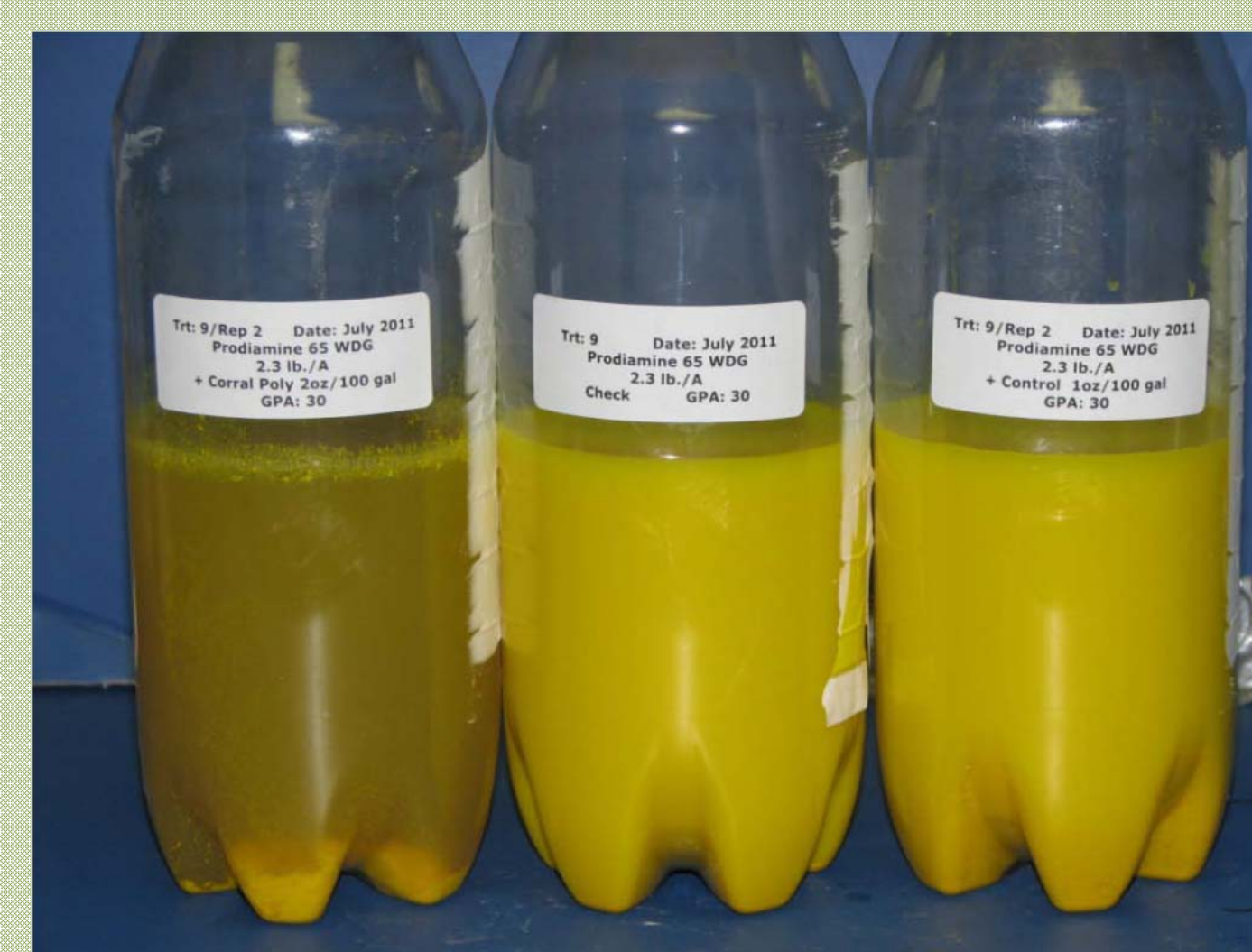
Figure 3. Bottle on left contains the incompatible mixture of the herbicide Prodiamine 65 WDG (active ingredient prodiamine) and Corral® Poly brand adjuvant. Middle bottle contains only Prodiamine 65 WDG herbicide in water. Bottle on the far right contains compatible mixture of Control™ brand adjuvant and the herbicide Prodiamine 65 WDG.
