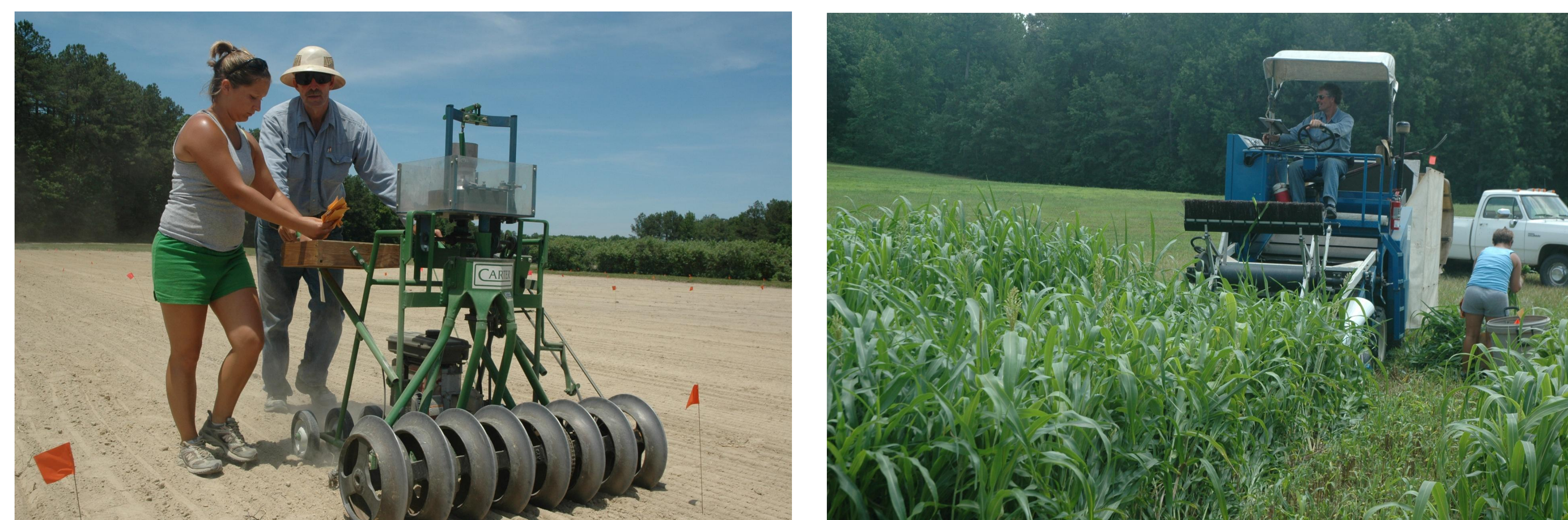
Figure 3. Plots were established with a cultipack type seeder (Carter Manufacturing, Brookston, IN) (left) and harvested with self-propelled sickle bar type forage harvester (Swift Machine, Swift Current, SK) (right).
