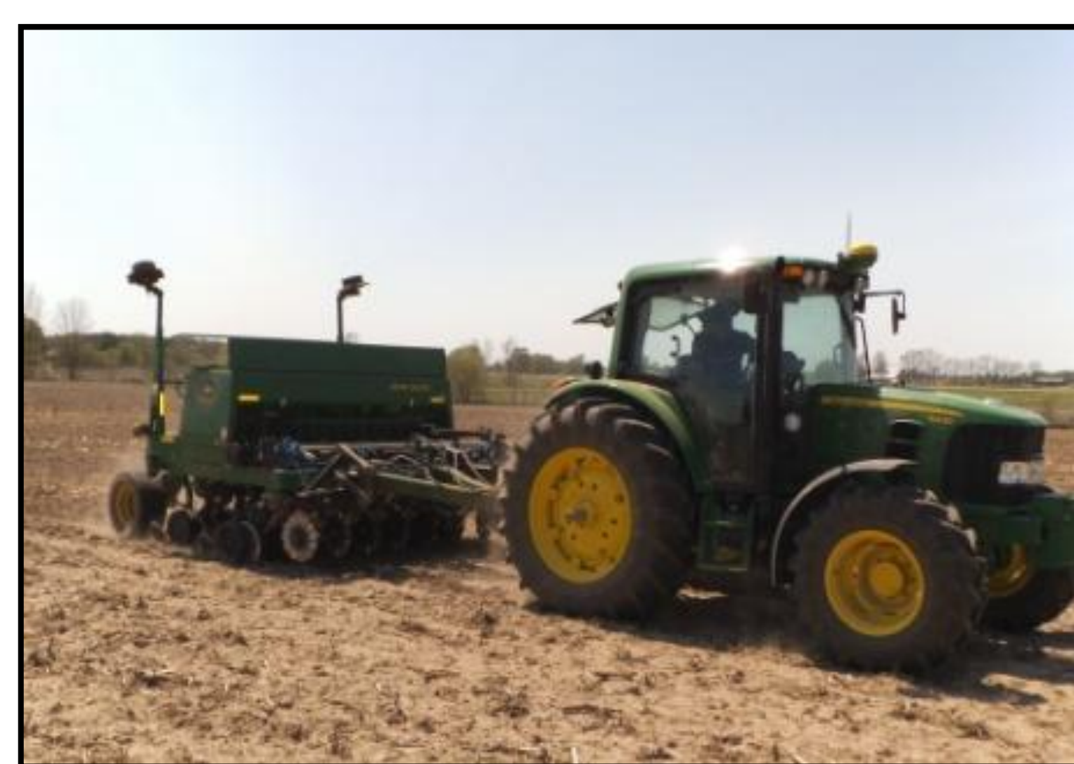
Figure 2. Seeding soybeans with a John Deere 1560 no-till drill
