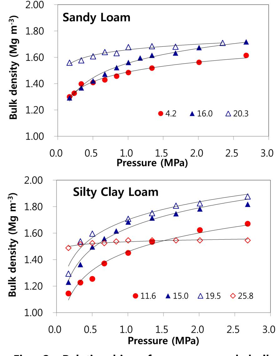
2. Relationship of pressure and bulk Fig. density for silty clay loam and sandy
