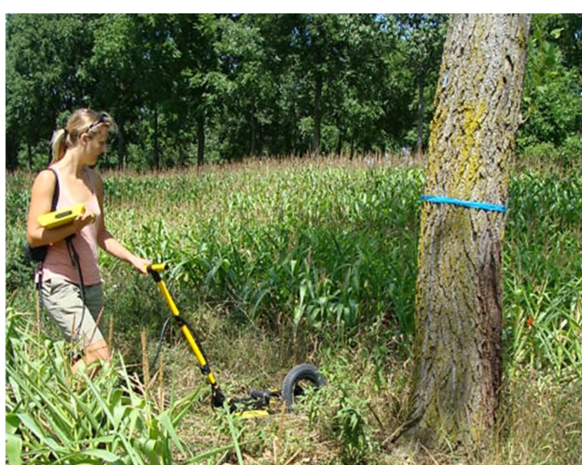
Figure 2. Collecting subsurface data using a 1000 MHz GPR in a tree-based intercropping system.
