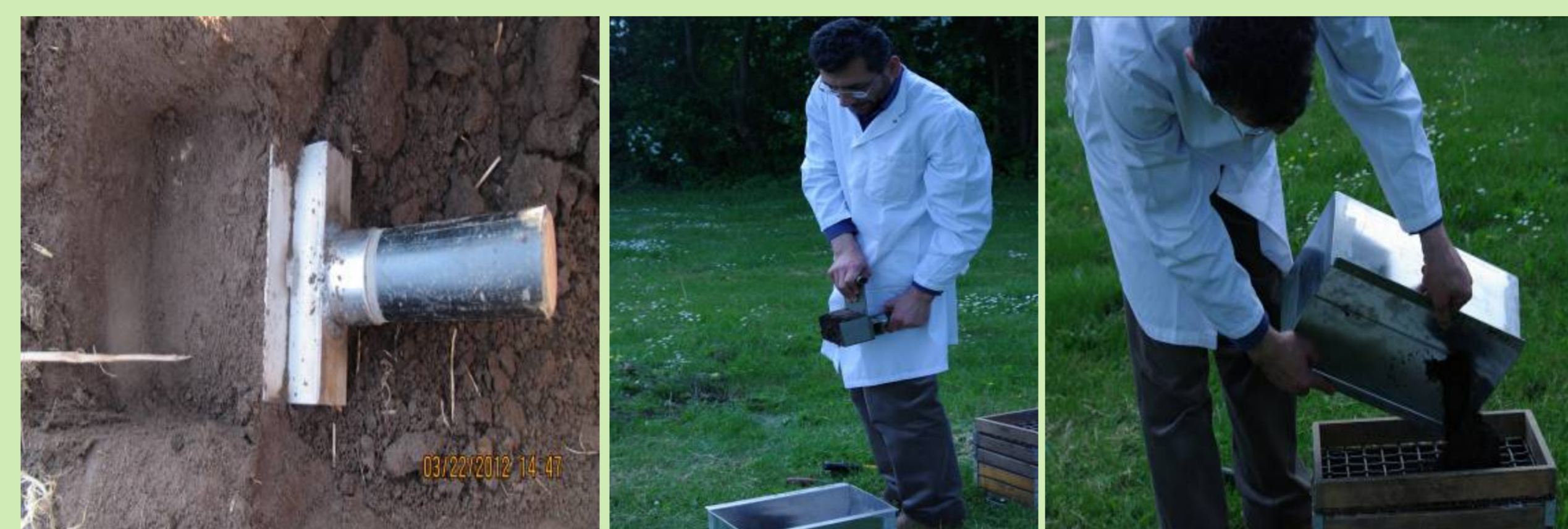
determined aggregate size distribution after a drop shatter test for soil taken from 10-20 cm depth (Schjønning et al. 2002)
