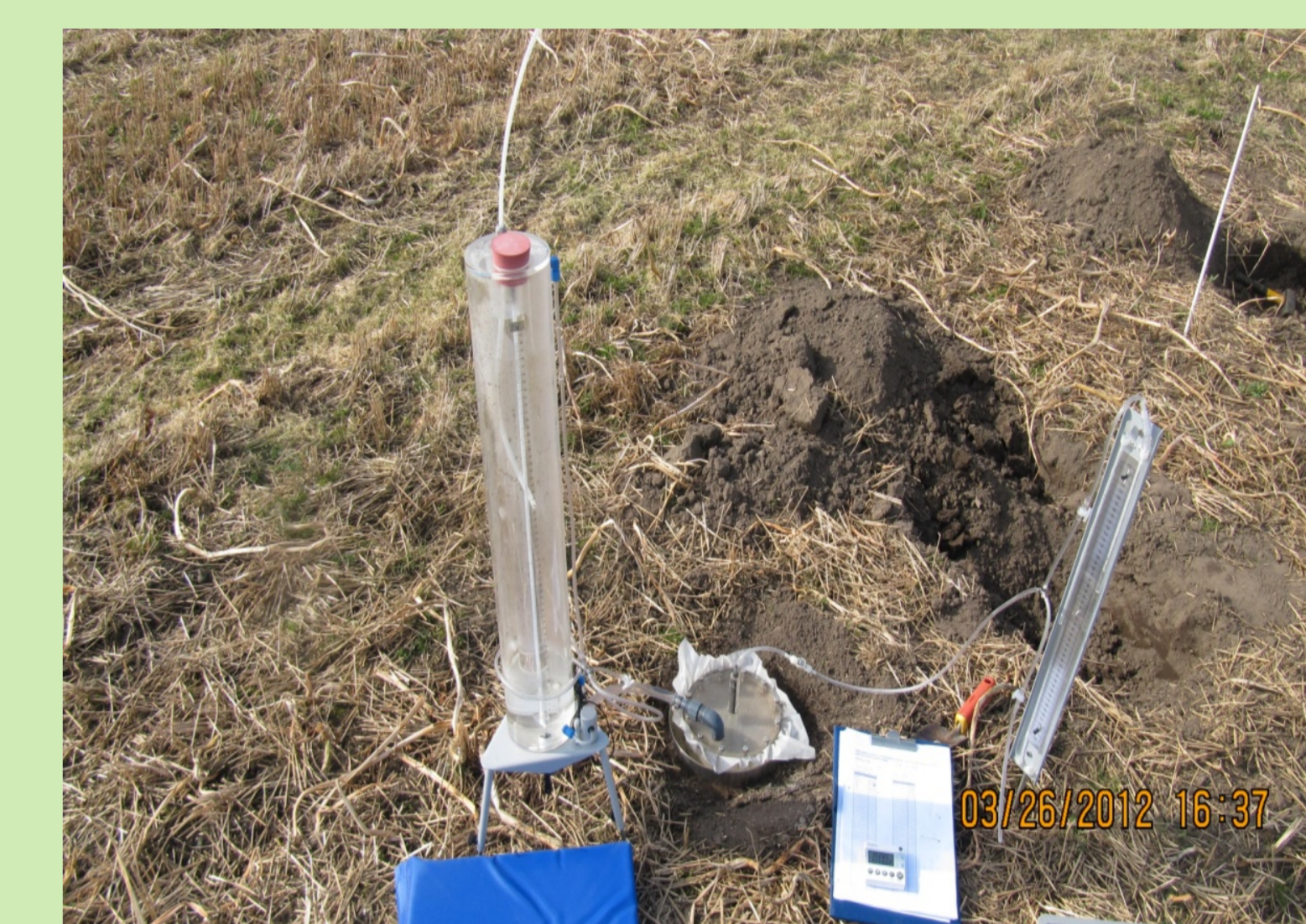
measuring unsaturated hydraulic conductivity at -4 hPa in field
