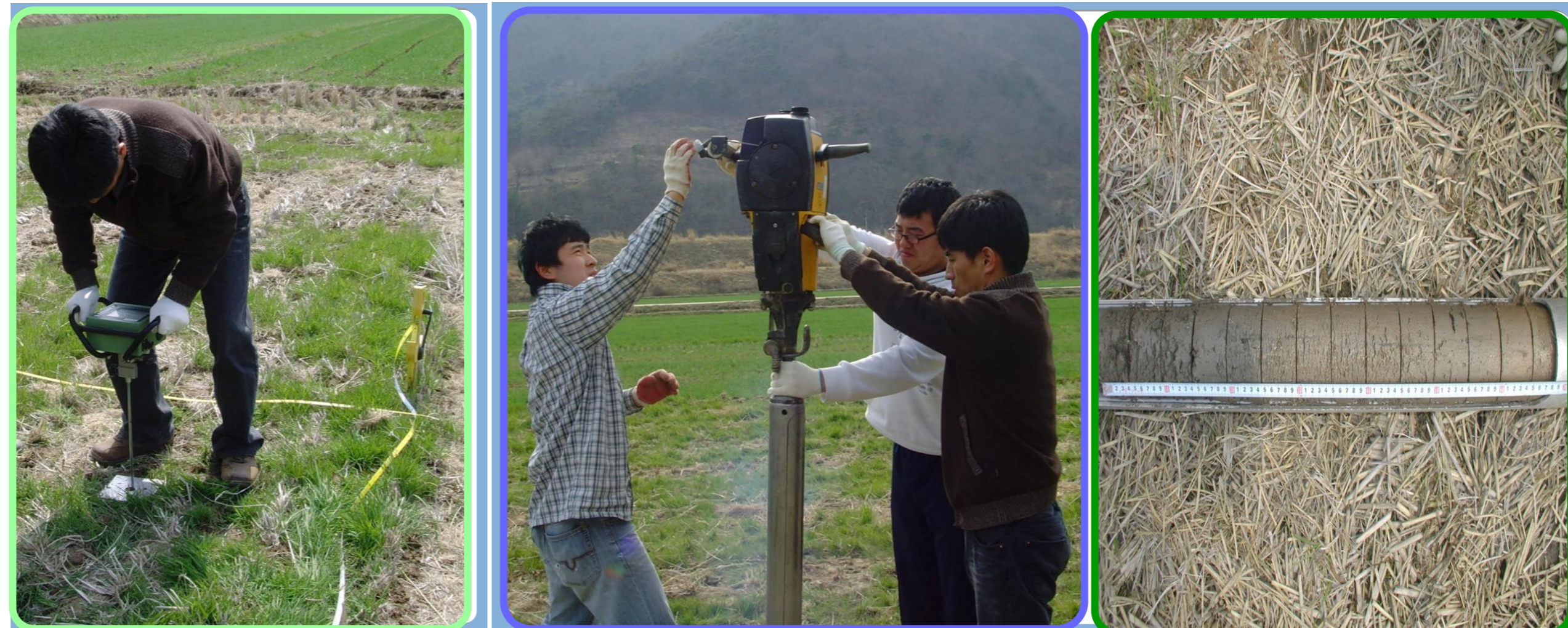
Photo 2. Measurement of cone index by digital cone penetrometer and segment of soil profile.
