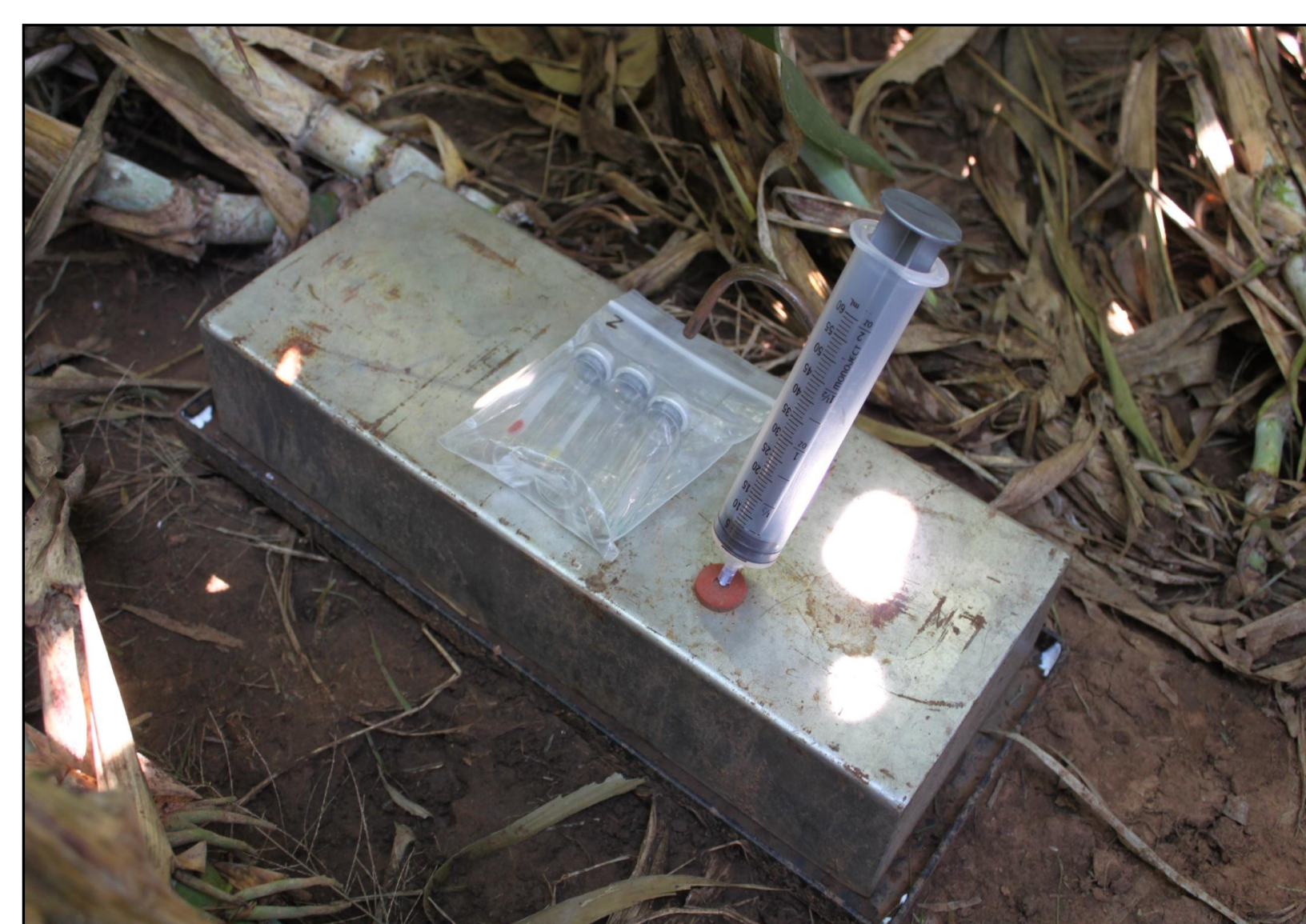
Figure 1: Parallel oriented chamber with sampling vials and syringe primed for sampling.
