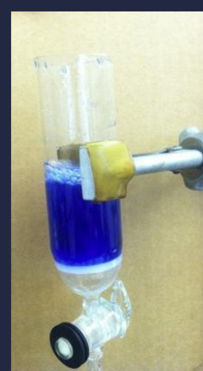
Figure 3. Glass frit apparatus with Remazol Brilliant Blue dye.
