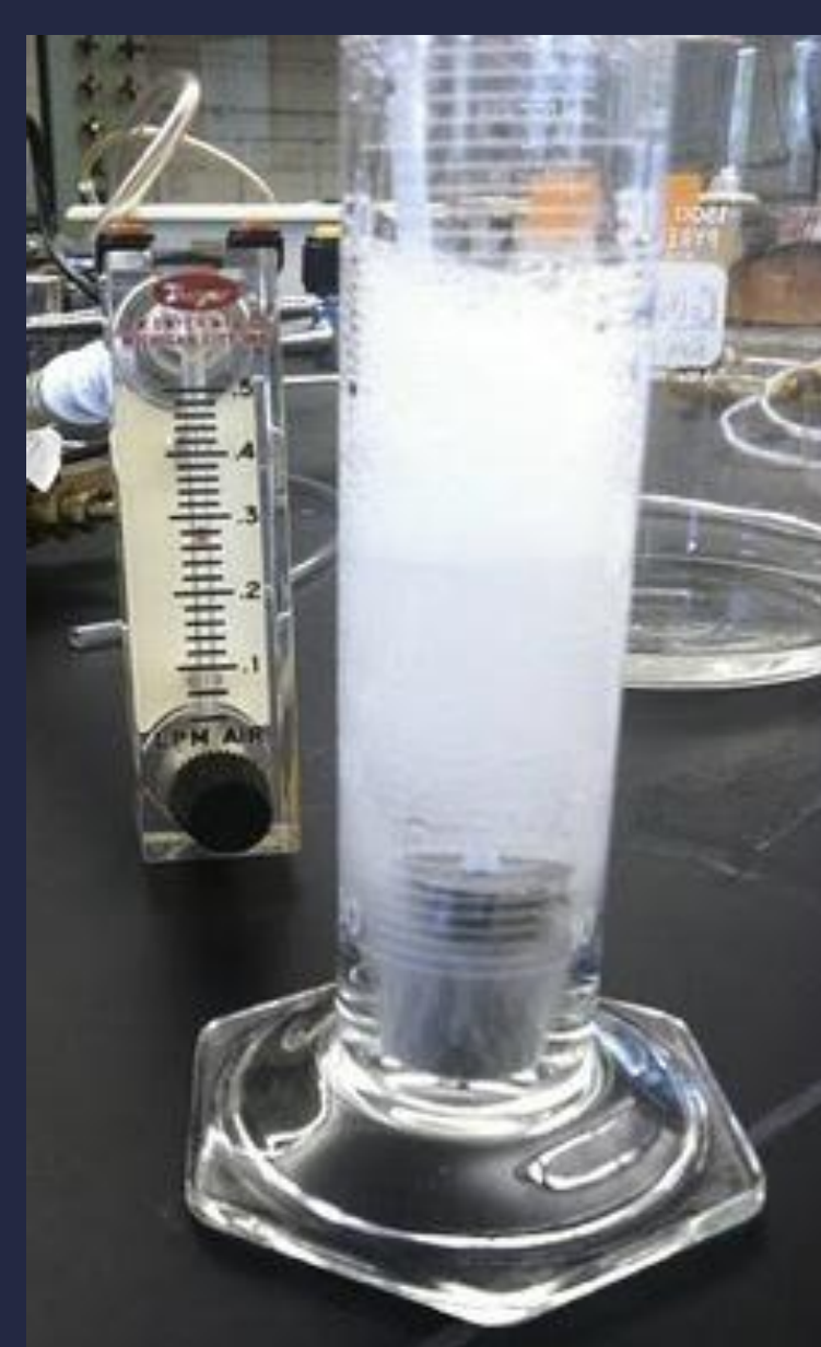
Figure 2. Introduction of ozonated air into water by a metal frit.
