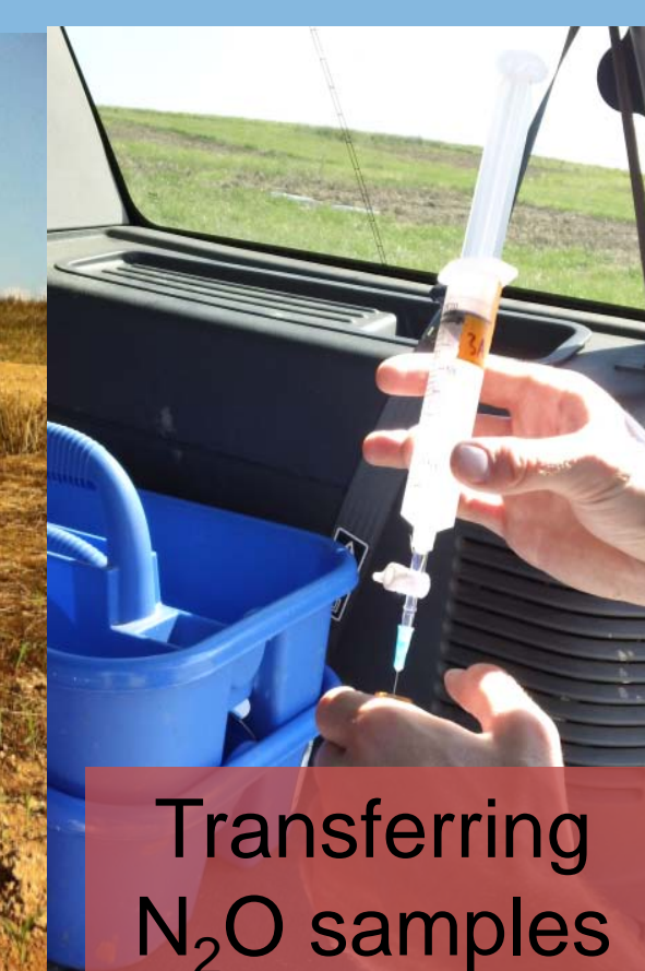
Gas sampling for GC analysis
