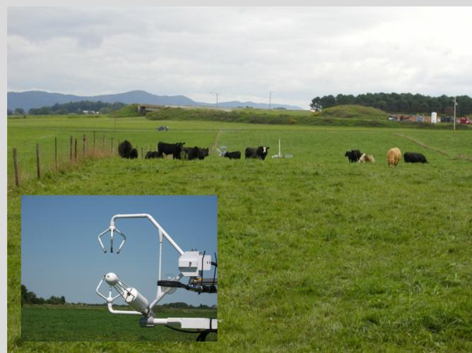
Micrometeorological techniques (eddy covariance) were used to examine the effect of N fertilization on carbon dioxide flux from two pastures in central Pennsylvania that were managed for grazing and hay production.
