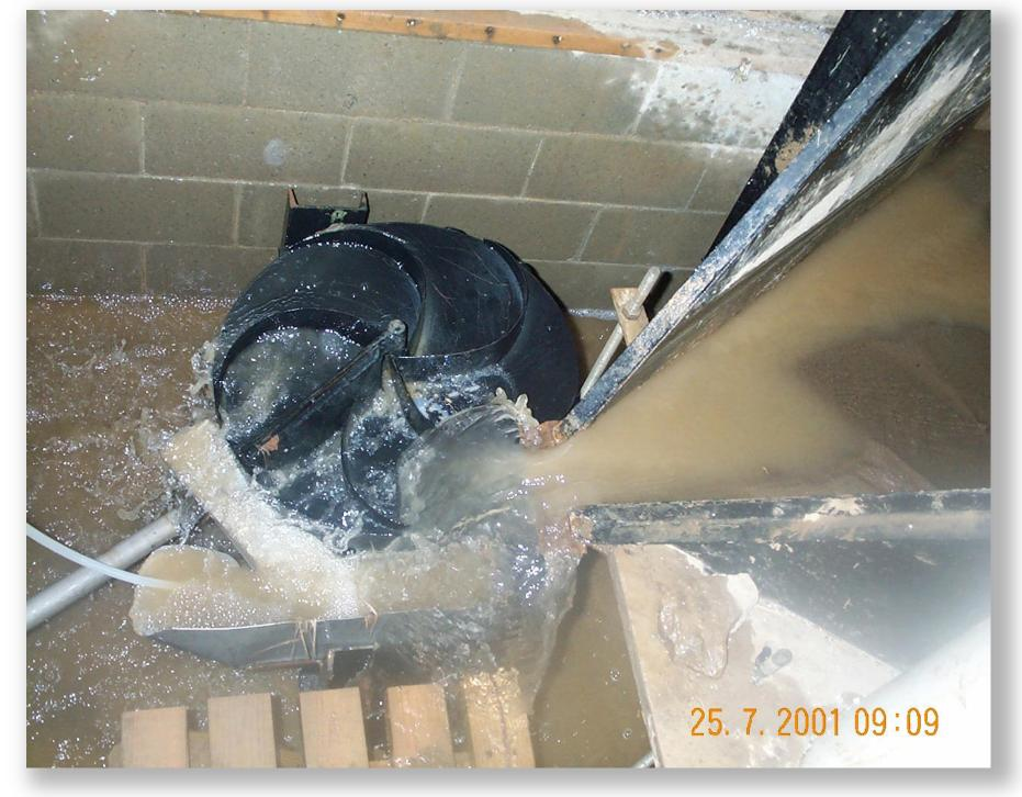
H-Flume and Coshocton Wheel Sampler
