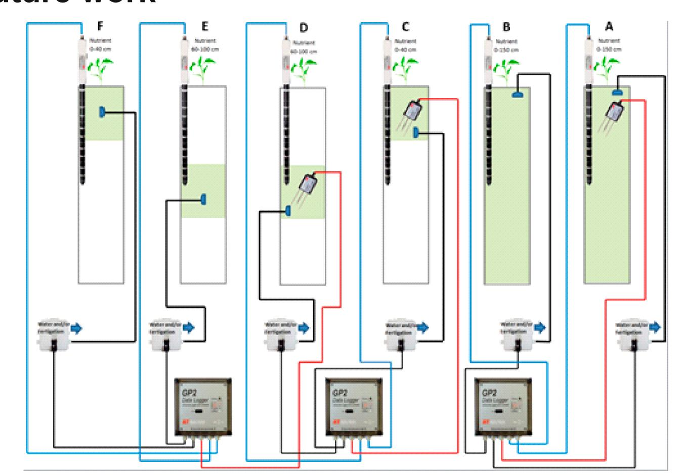
The next step in this experimental investigation will be to employ Delta-T's GP2 Advanced Logger and Controller with the WET Sensor and the PR2 Profile Probe to measure and log soil conductivity (nutrient level), soil moisture and temperature. Each GP2 is capable of providing precise closed-loop irrigation control at different soil depths when combined with the PR2, as well as fertigation control when combined with the WET Sensor.
