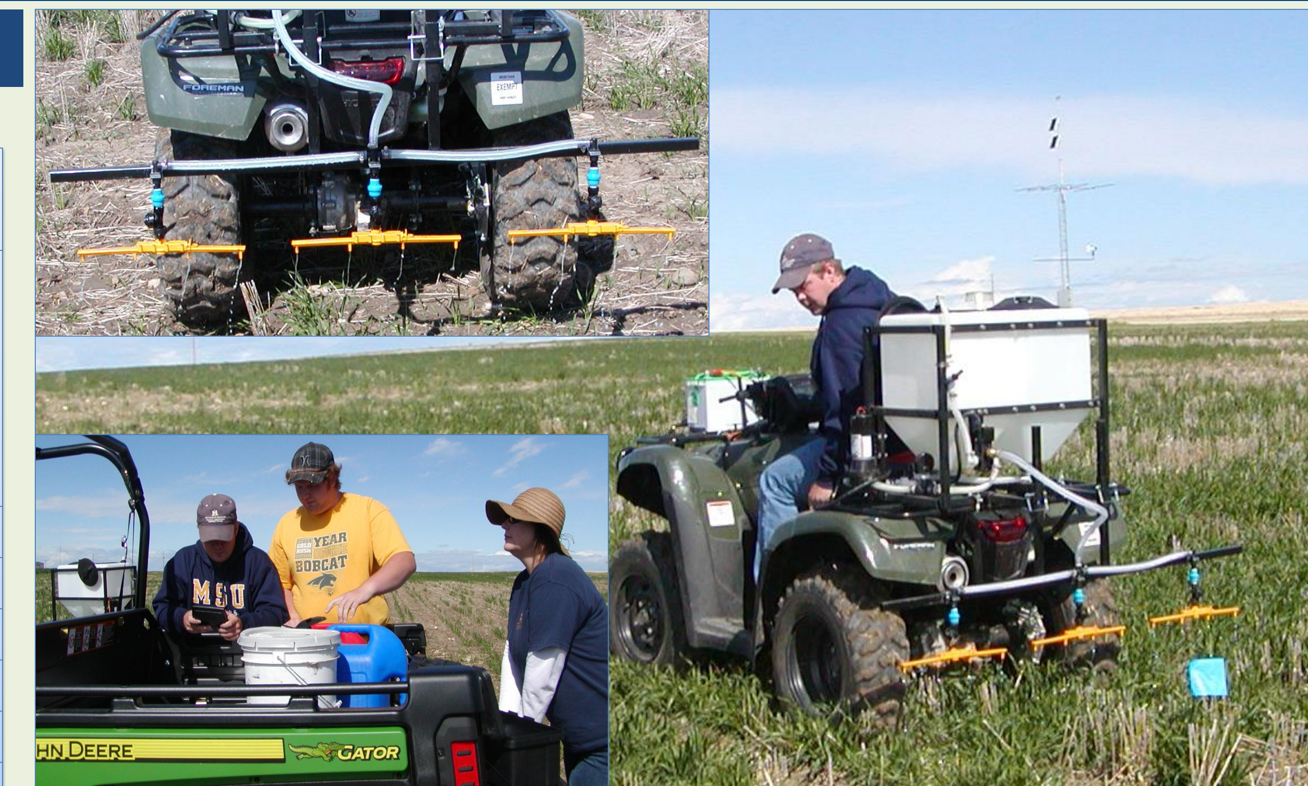
Applying foliar N fertilizers to spring wheat plots using an ATV-mounted stream bar sprayer, Montana, 2012
