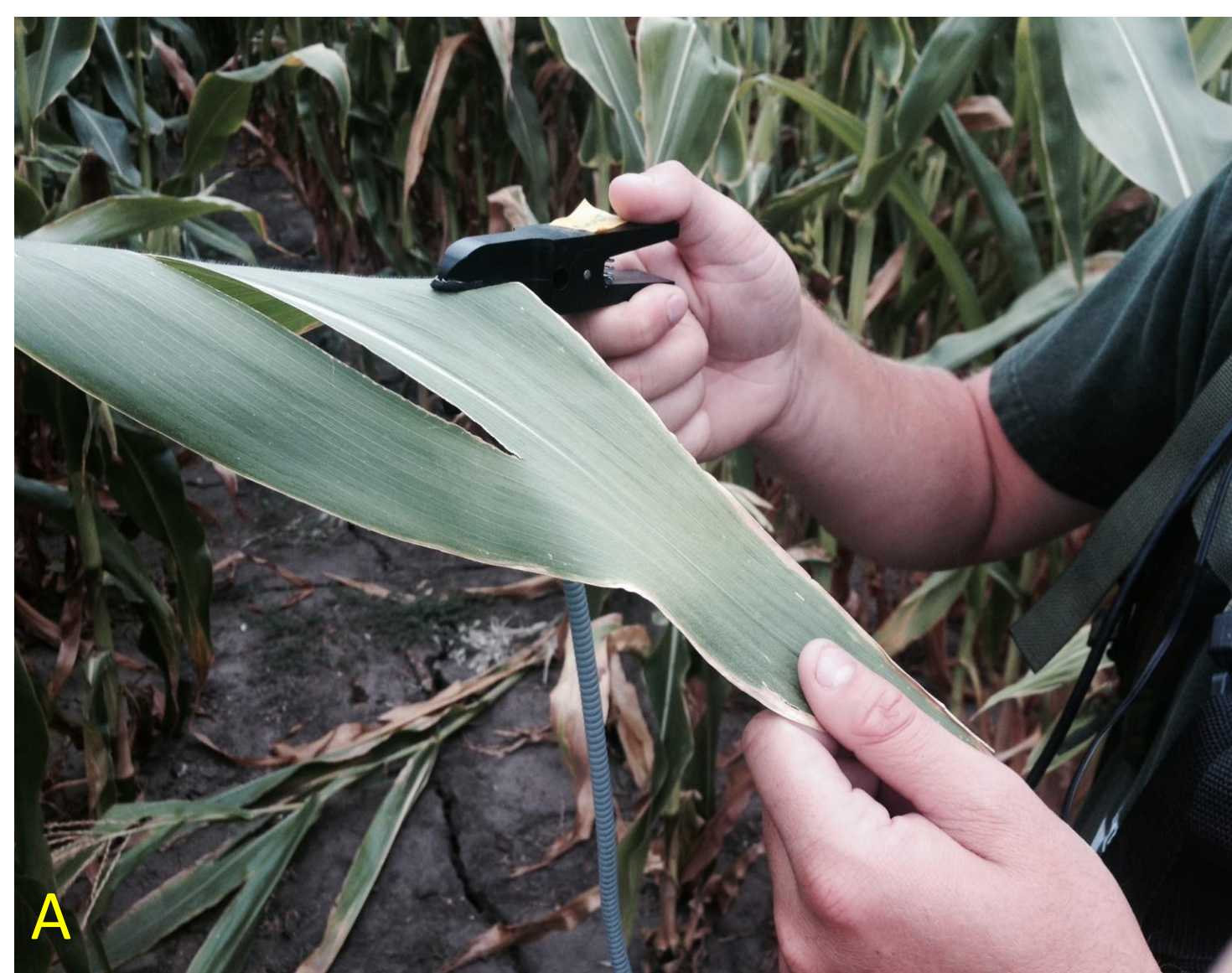
Figure 1. High-throughput phenotyping technology. A) The leaf clip position on a leaf. B) The hyperspectral backpack system attached to the leaf clip.
